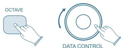
*NOTE: The (Transpose/Octave) Button will remain lit while active. To deactivate (Transpose/Octave), simply press the button and the Allegro will return to its default configuration.*
